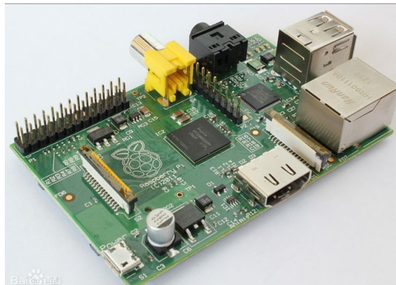
Figure 12: Raspberry Pi Board
